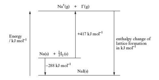
Use the information given to calculate the enthalpy change of lattice formation (in kJ mol<sup>-1</sup>) of sodium iodide. [2]
